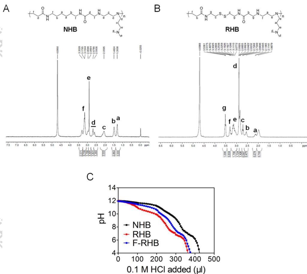
**Figure 2.** Physicochemical characterization of polymers. <sup>1</sup>H NMR spectra of NHB (A) and RHB (B). (C) Acid–base titration curves. Volume of HCl used to adjust the pH value of the polymer solutions from pH 12 to 4. (NHB, nonbio-reducible hyperbranched poly(amido amine); RHB, bio-reducible hyperbranched poly(amido amine)).
