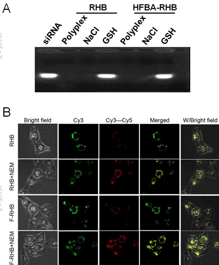
**Figure 4.** Reduction-triggered disassembly of polyplexes. (A) Reduction-triggered siRNA release from RHB and F-RHB polyplexes analyzed by agarose gel electrophoresis. (B) FRET analysis of GSH-triggered intracellular disassembly of polyplexes prepared from a mixture of Cy3-siRNA and Cy5-siRNA.
